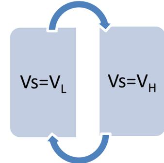
$$V_e \geq \frac{R_1}{R_1+R_2} V_H = k_i V_H$$
