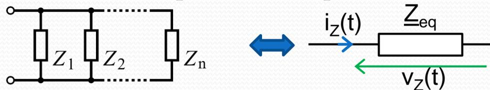
$$\frac{1}{\underline{Z_{eq}}} = \frac{1}{\underline{Z_1}} + \frac{1}{\underline{Z_2}} + \dots + \frac{1}{\underline{Z_n}}$$
