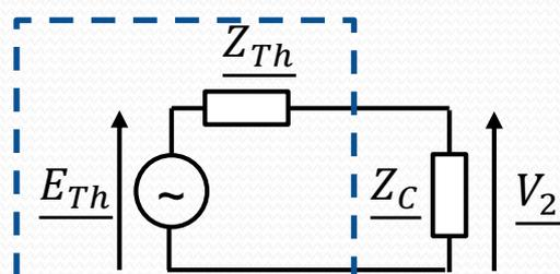
$$\underline{E}_{Th} = \frac{V_1 \cdot \underline{Z}_2}{\underline{Z}_1 + \underline{Z}_2}; \quad \underline{Z}_{Th} = \frac{\underline{Z}_1 \cdot \underline{Z}_2}{\underline{Z}_1 + \underline{Z}_2}$$
