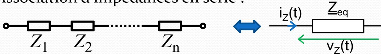
$$\underline{Z_{eq}} = \underline{Z_1} + \underline{Z_2} + \dots + \underline{Z_n}$$
