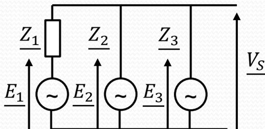
$$\underline{V}_S = \frac{\frac{\underline{E}_1}{\underline{Z}_1} + \frac{\underline{E}_2}{\underline{Z}_2} + \frac{\underline{E}_3}{\underline{Z}_3}}{\frac{1}{\underline{Z}_1} + \frac{1}{\underline{Z}_2} + \frac{1}{\underline{Z}_3}}$$
